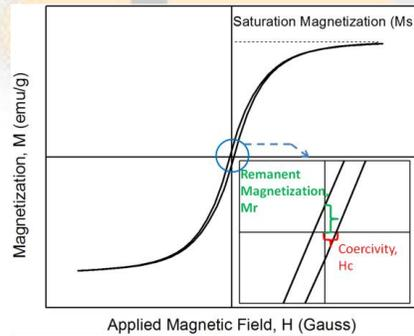
Figure 1. Magnetization versus applied magnetic field loop depicting saturation magnetization Ms, remanent magnetization Mr and Coercivity, Hc of soft ferrite.
